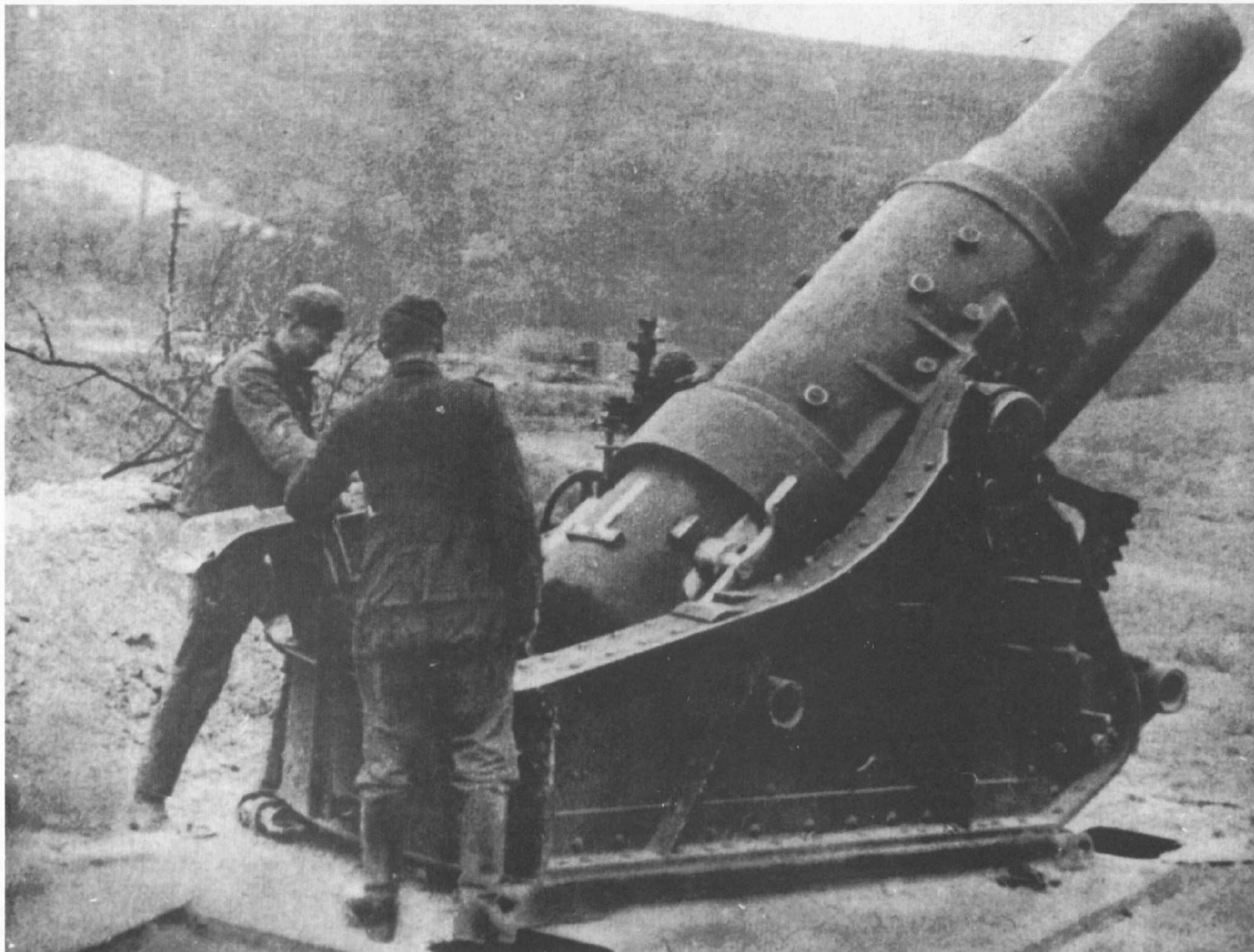
The 30.5 cm mortar (t) could fire 289-kilogram shells to a distance of 12,300 meters, and was especially good for attacking fortresses. 21 guns were used in June 1942 in Operation "Störfang" (the capture of the Sevastopol fortifications) in Crimea.
