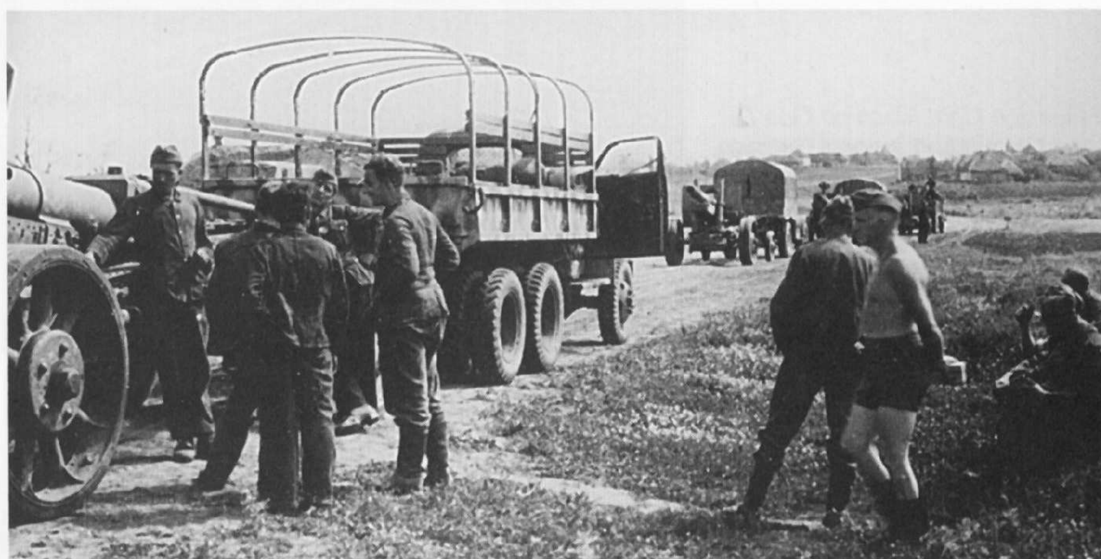
A Light Artillery Tractor 601 (r)-russ. CT-3- tows the staff bus of an army unit through rough terrain. Large numbers of Stalinez tractors were also used for such purposes.
