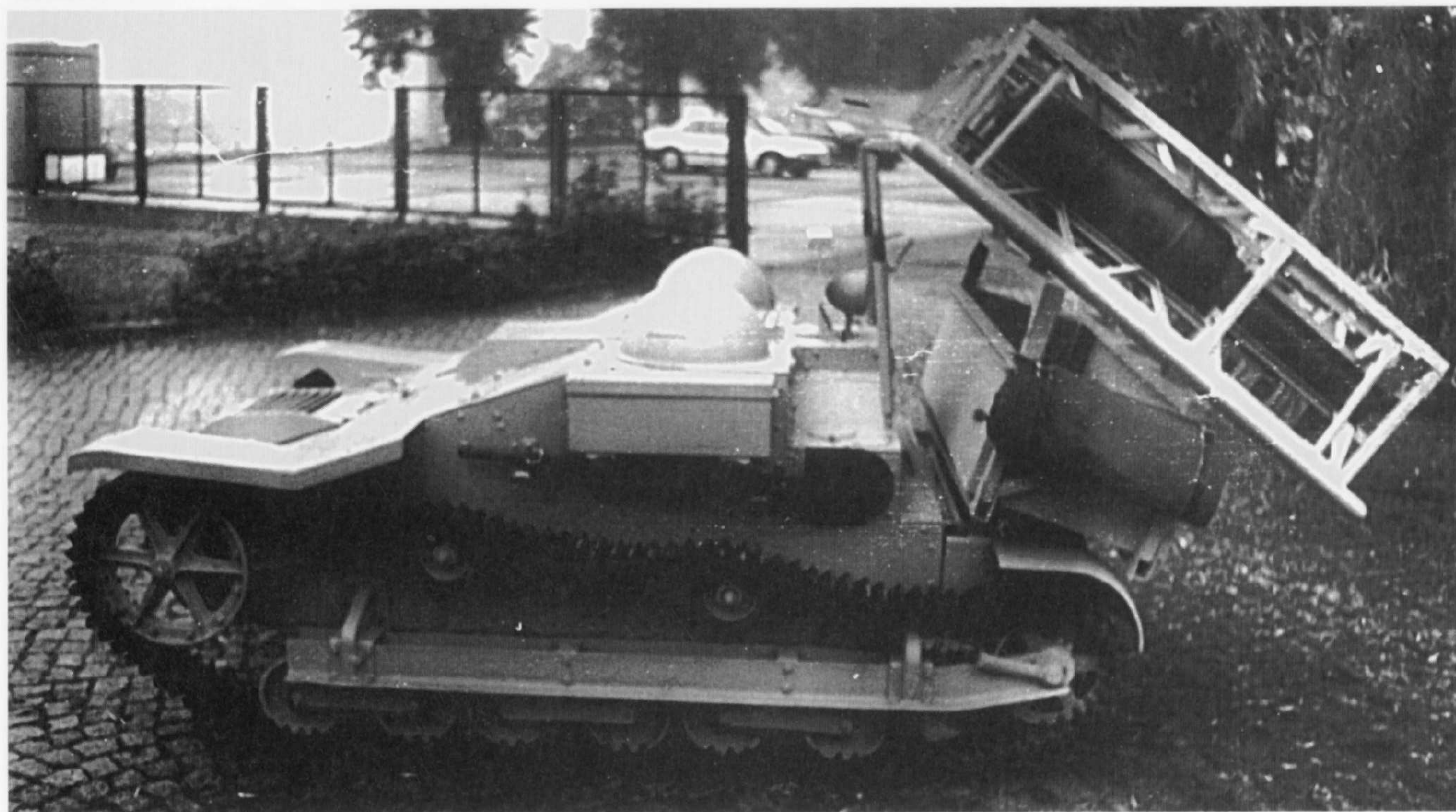
Above and below: In 1944, Field Marshal Rommel took up a suggestion from the 21st Panzer Division to produce improvised salvo guns in order to attack the landing attempts in the west at sea. This resulted in, among others, the Infantry Tractor UE 630 (f) with the 28/32 cm Launcher 41.
