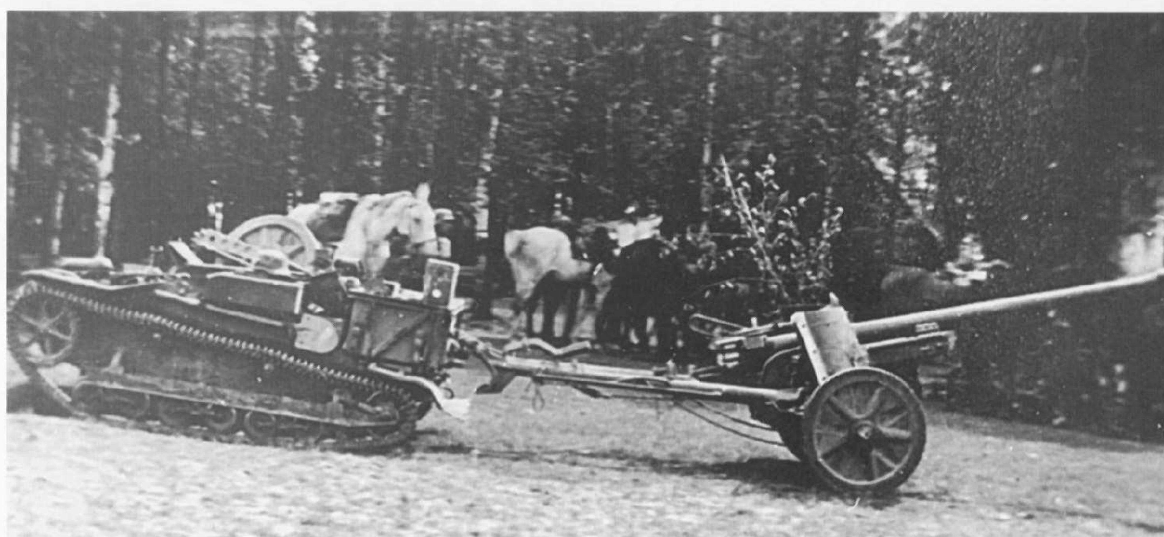
Right: This UE 630 (f) armored ammunition carrier tows a 5 cm Panzerjäger Cannon 38 for an Infantry Panzerjäger company on the eastern front, in the summer of 1941.
