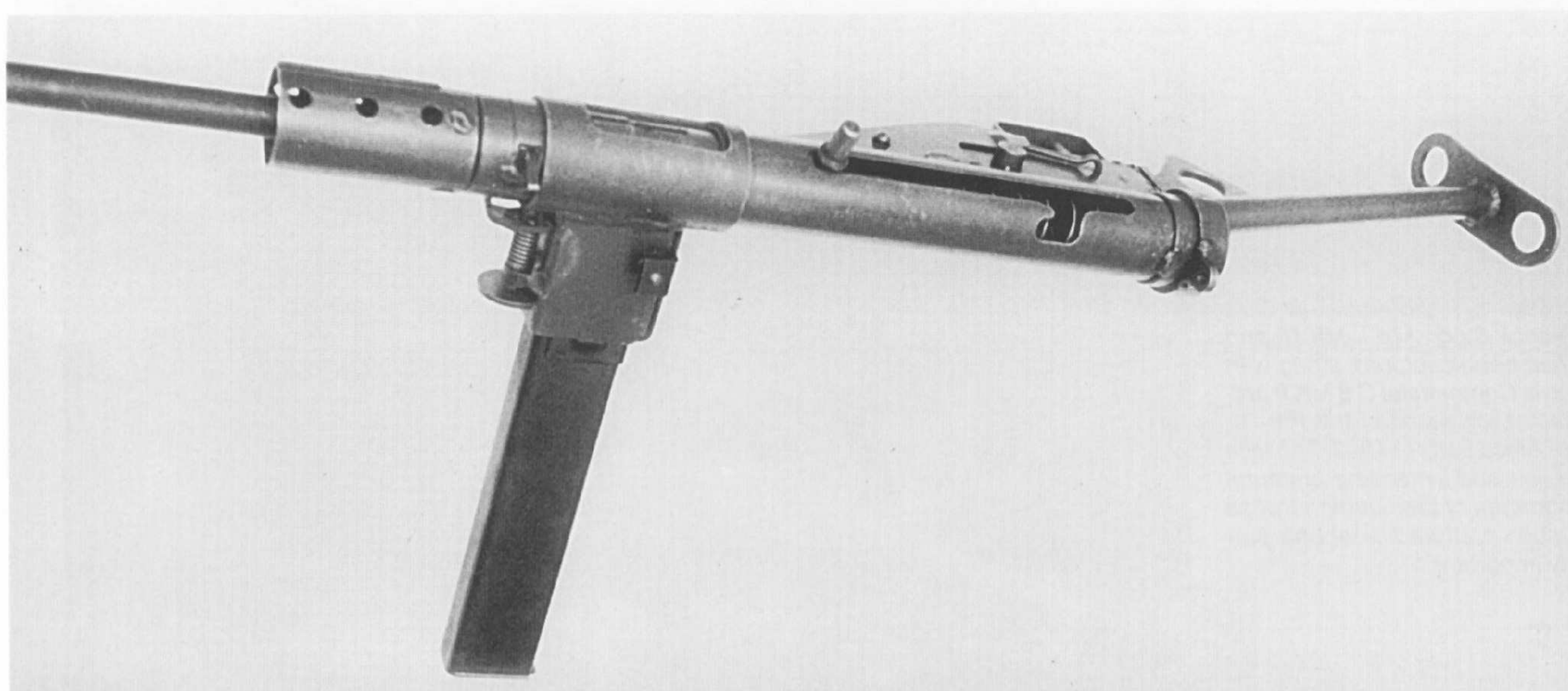
The STEN Mk. II Machine Pistol 749 (e)-engl. was captured in large numbers by the Germans, along with sabotage weapons. This gun could also fire German-made 9 mm ammunition, and was rebuilt and turned over to the Volkssturm toward the end of the war.
