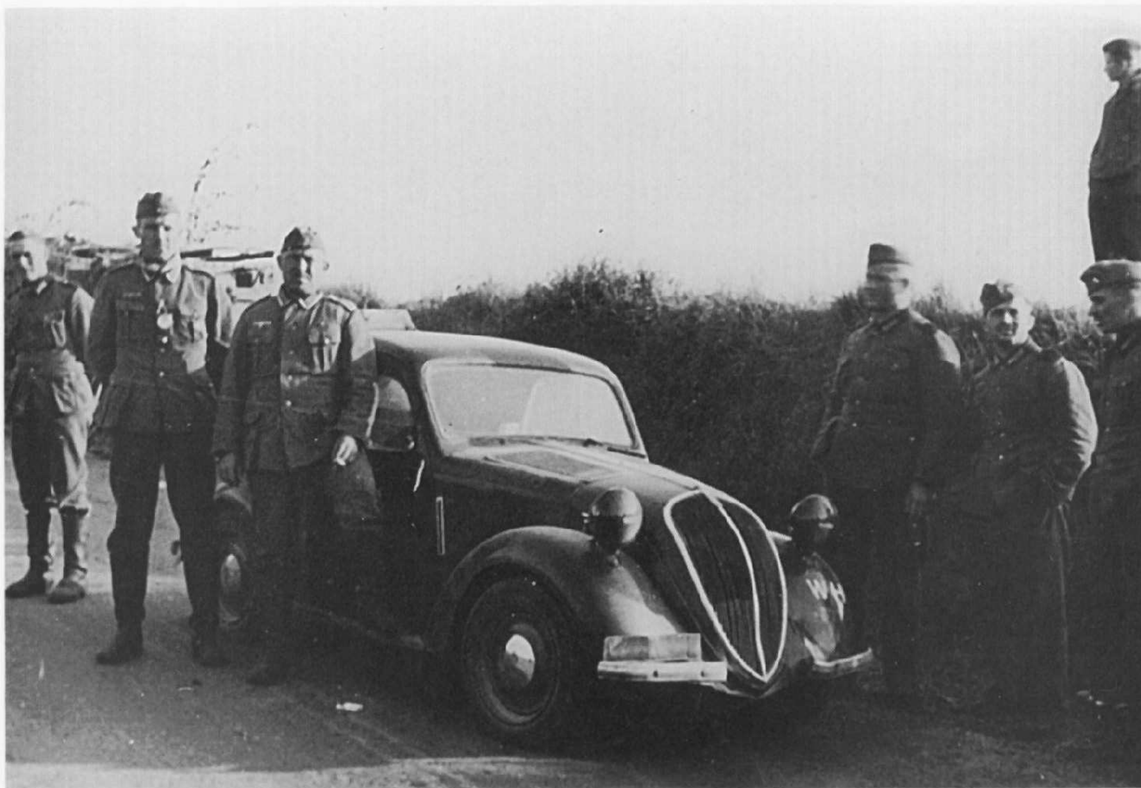
The Simca Cinq car was taken over from French military stocks. The car, with a 13 HP engine, was not up to the rough conditions of front-line use. It lasted longer with training and replacement units.
