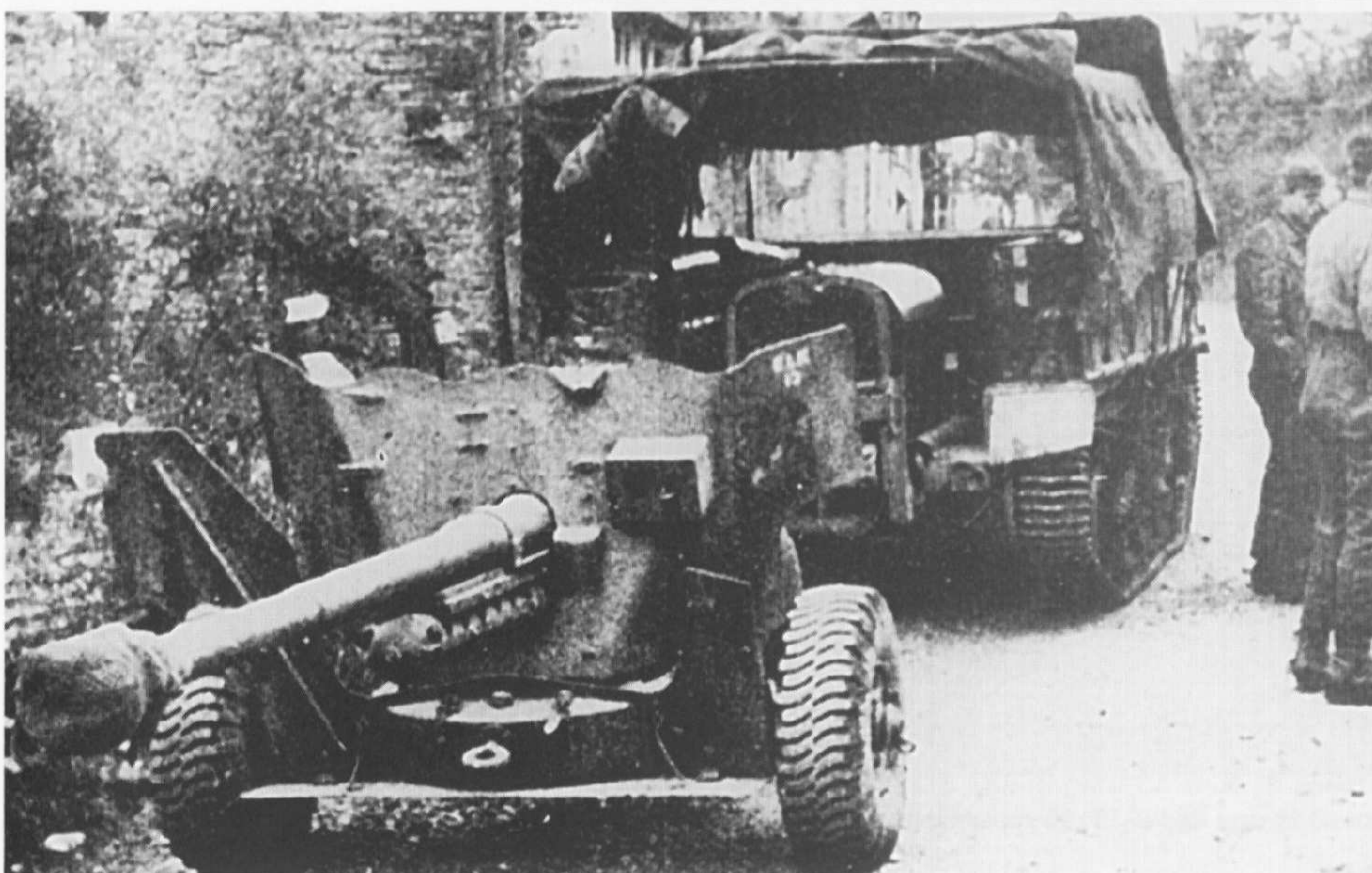
This 5.7 cm Antitank Gun 209 (e)-engl. 6 pdr. MK III- was captured from the British in Normandy early in July 1944. A Lloyd Carrier is towing it.
