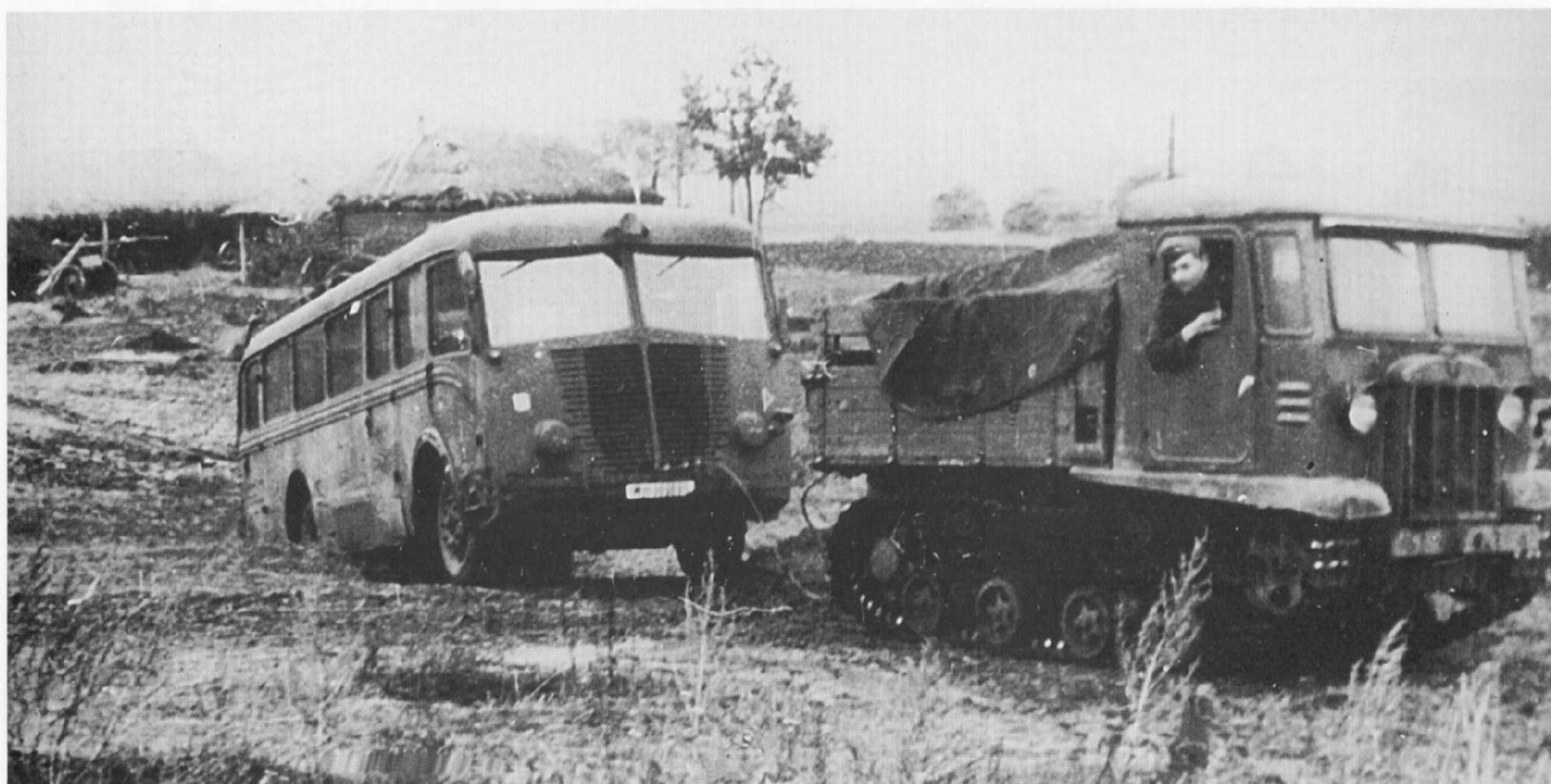
A Light Artillery Tractor 601 (r)-russ. CT-3- tows the staff bus of an army unit through rough terrain. Large numbers of Stalinez tractors were also used for such purposes.
