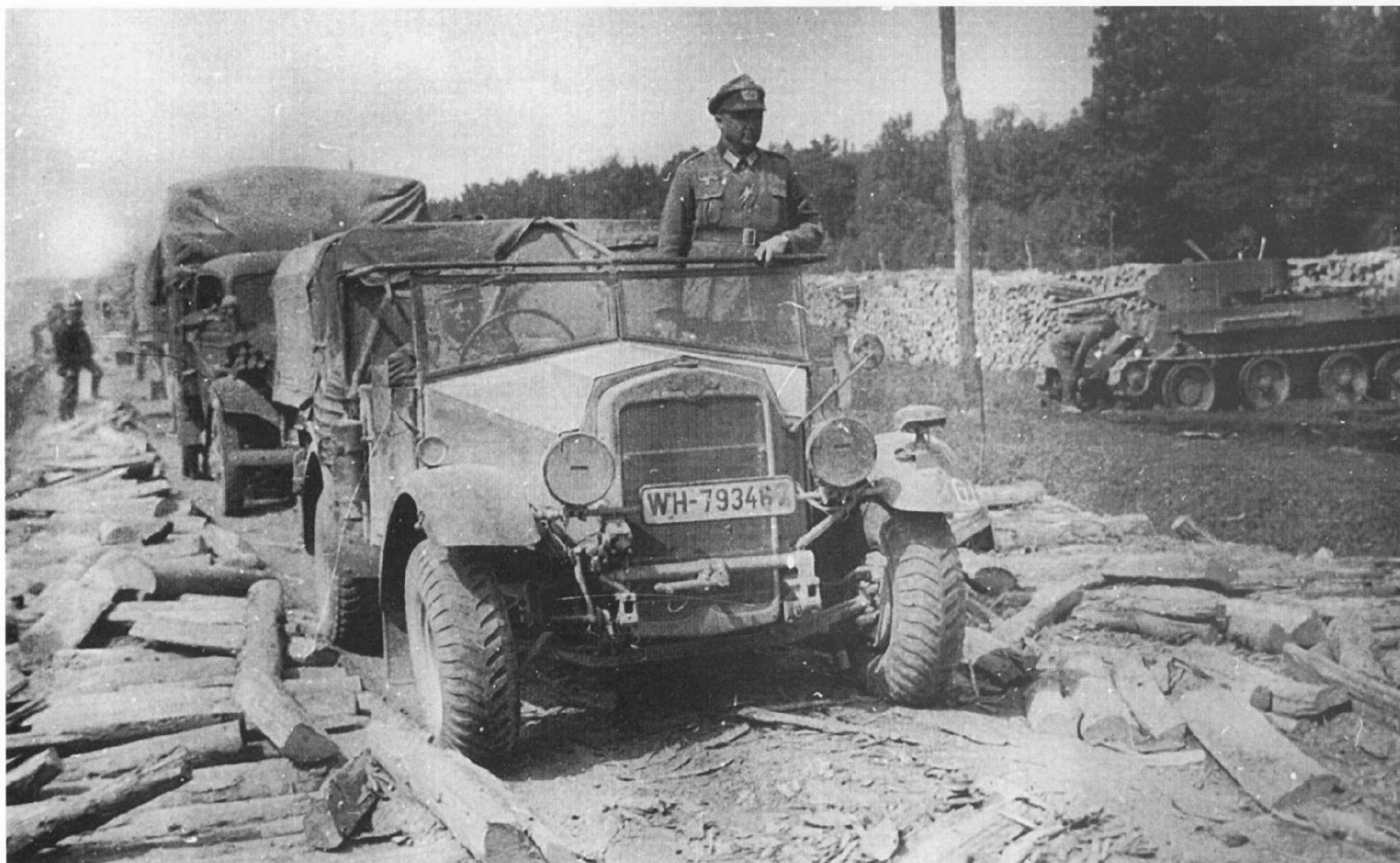
Robust and reliable: a British 15 cwt Morris Commercial CS-8 (4x2) truck used as a German unit's command vehicle on the eastern front in July 1941.
