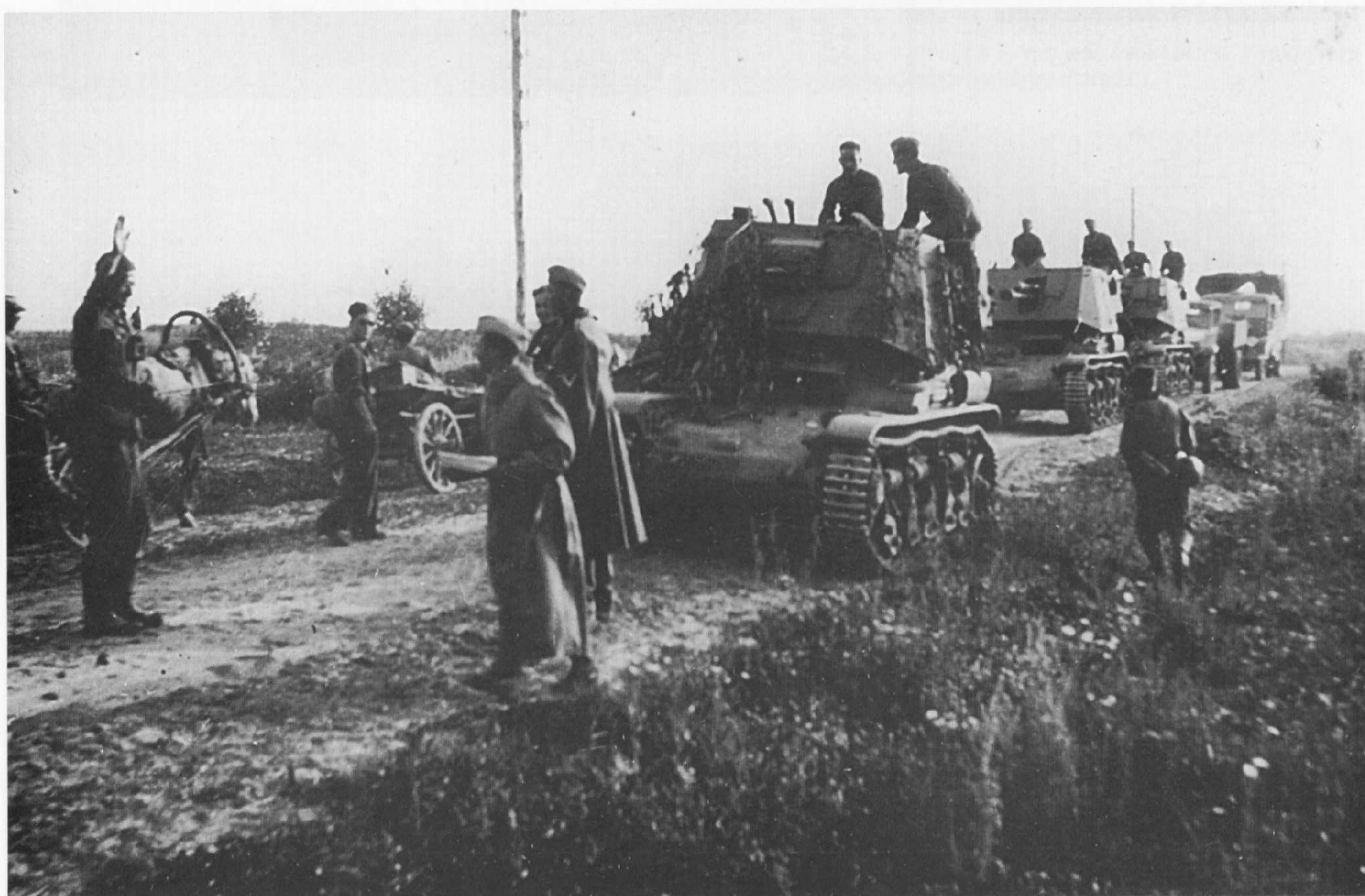
Between May and October 1941, the Alkett firm mounted 174 4.7 cm Pak (t) guns on R 35 (f) tanks as tank destroyers and rebuilt another 26 as command cars. The vehicles were used by, among others, Army Panzerjäger Unit 561. This picture shows a command car with MG 34 in a Ball Mantlet 30, followed by two tank destroyers with 4.7 cm guns.
