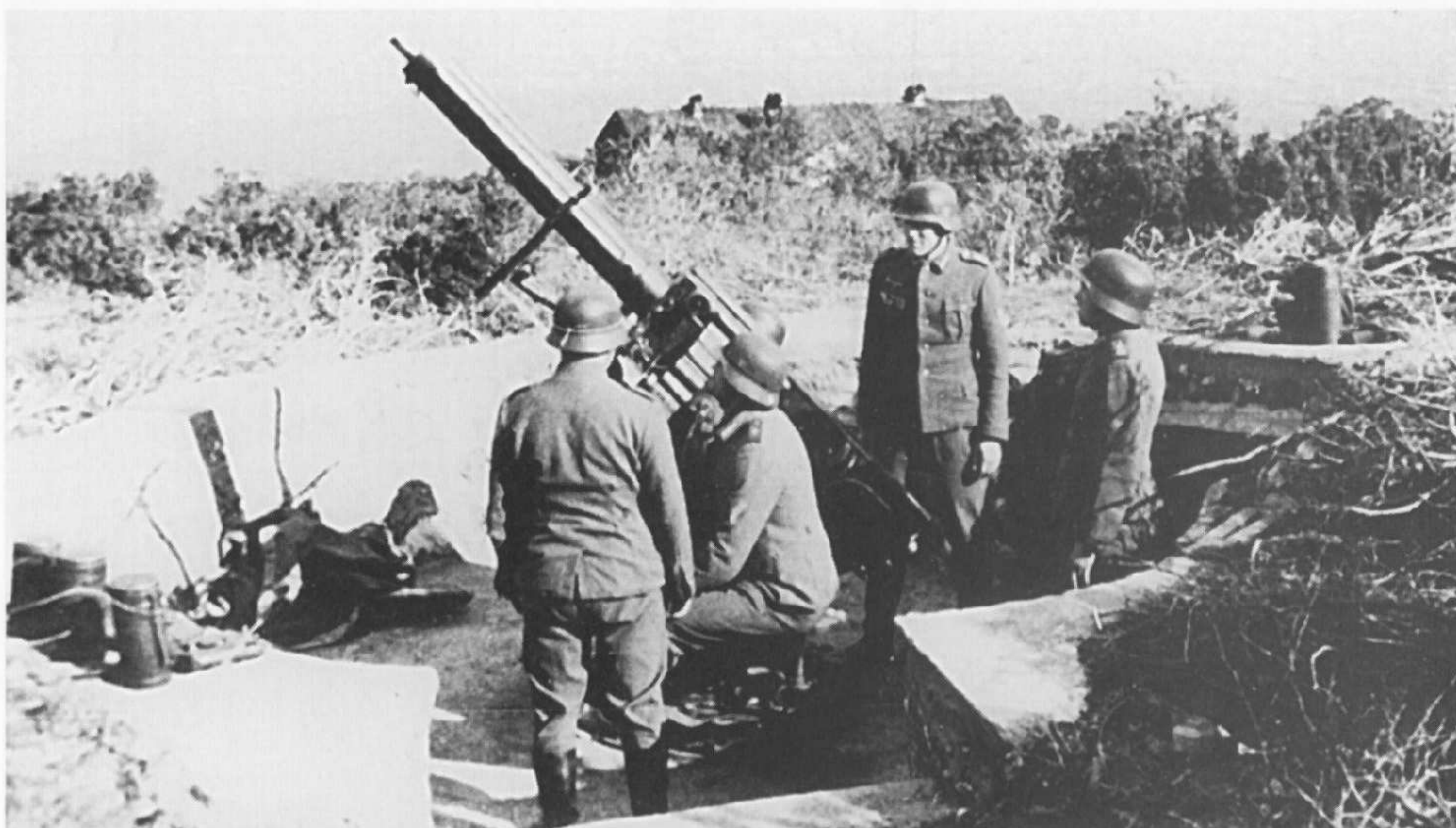
A weapon that came from British World War I supplies was the 4 cm Vickers anti-aircraft gun of 1918. The rate of fire was about 100 rounds per minute. This picture was taken on the French Atlantic coast in 1943.
