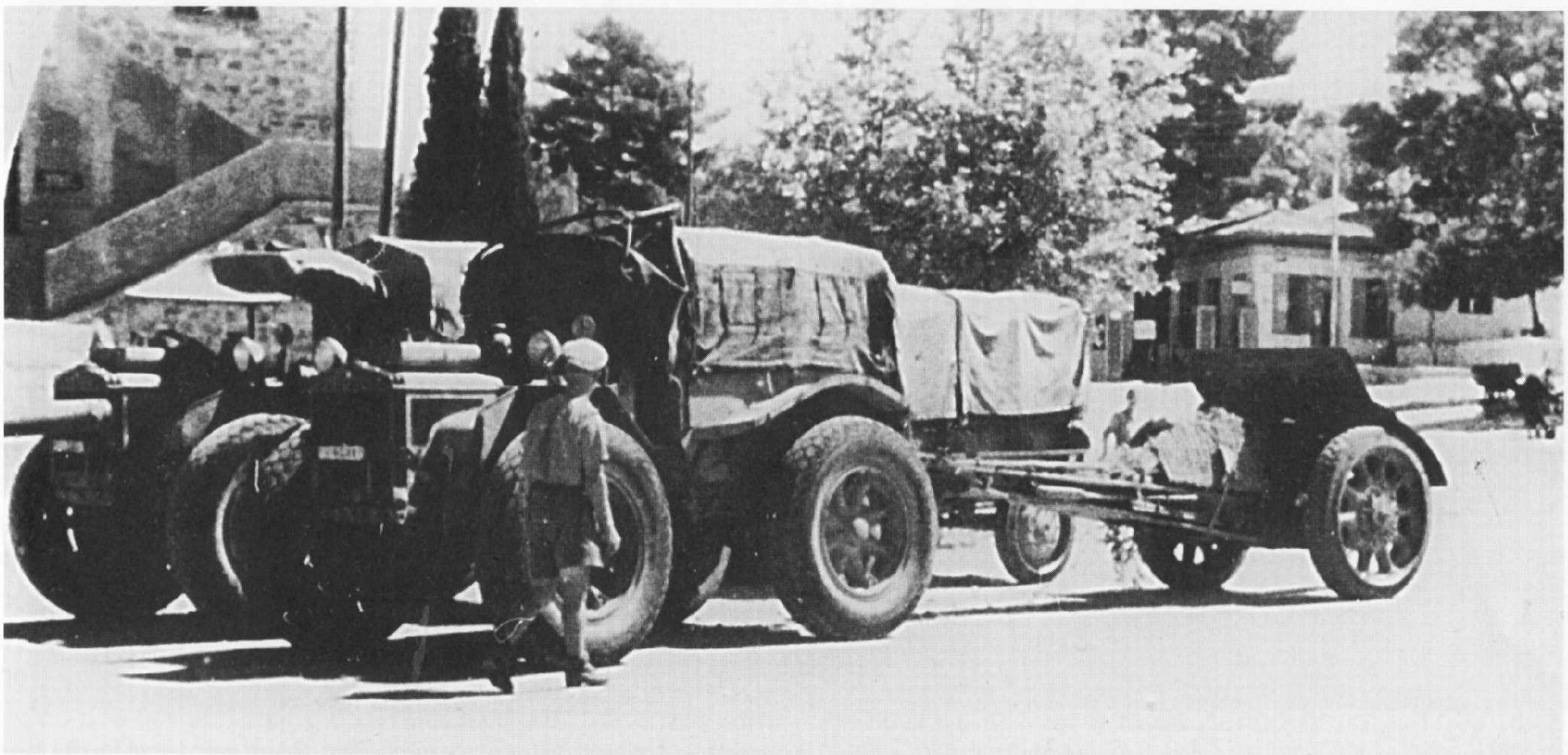
Two Fiat-Spa Pavesi P 4-110 heavy artillery tractors, one towing a 75 mm Field Cannon 237 (i) (Italian 75/27 M.06); the second tractor has an ammunition trailer in tow. They were taken over by a Navy command at a support point in Greece and photographed in September 1943.
