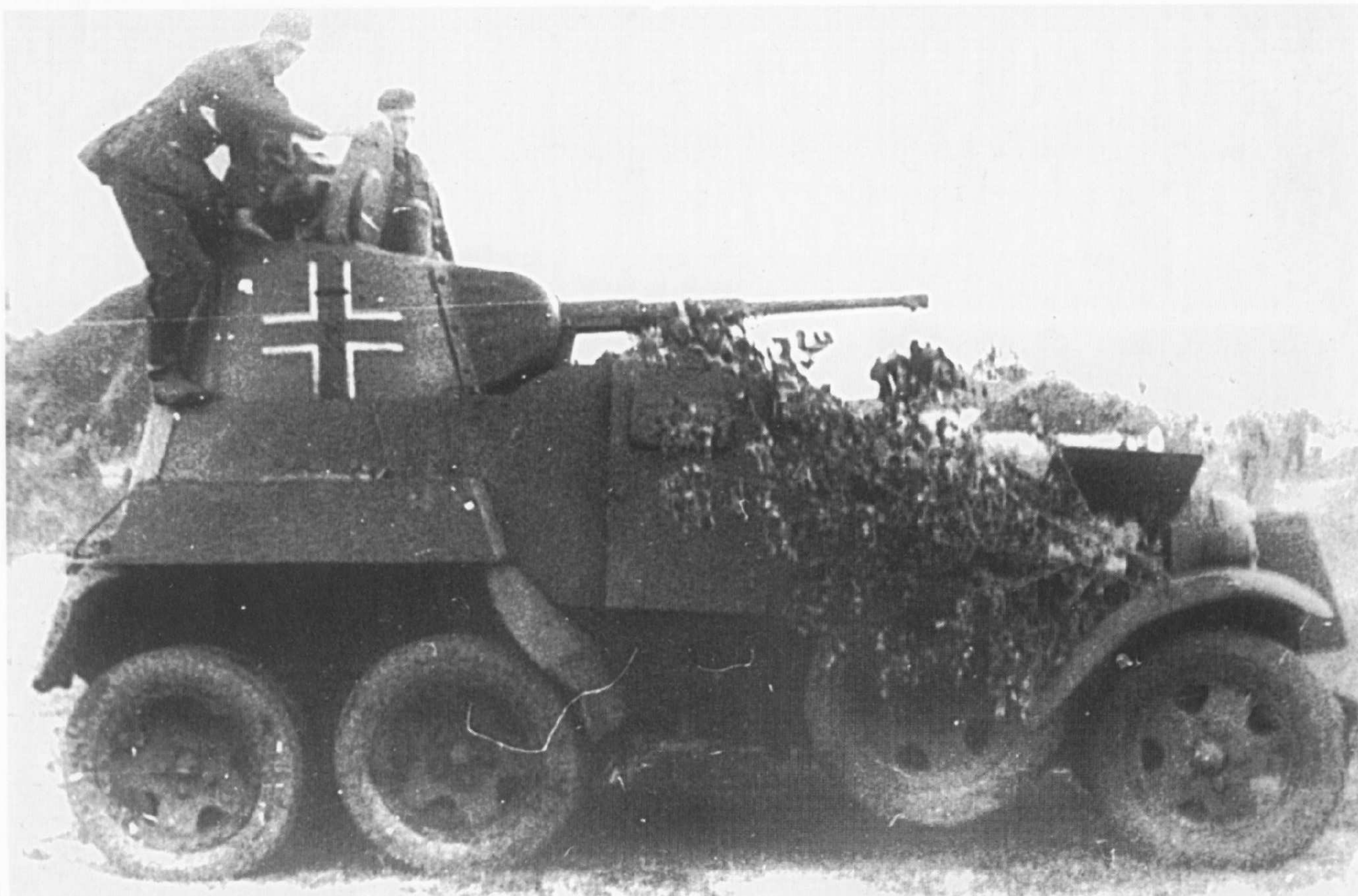
This light Armored Scout Car 203 (r), a Russian BA Ford, saw service in the east with the 14th Panzer Division. Its armament of one 45 mm Kampfwagenkanone and two machine guns gave the vehicle a respectable firepower.
