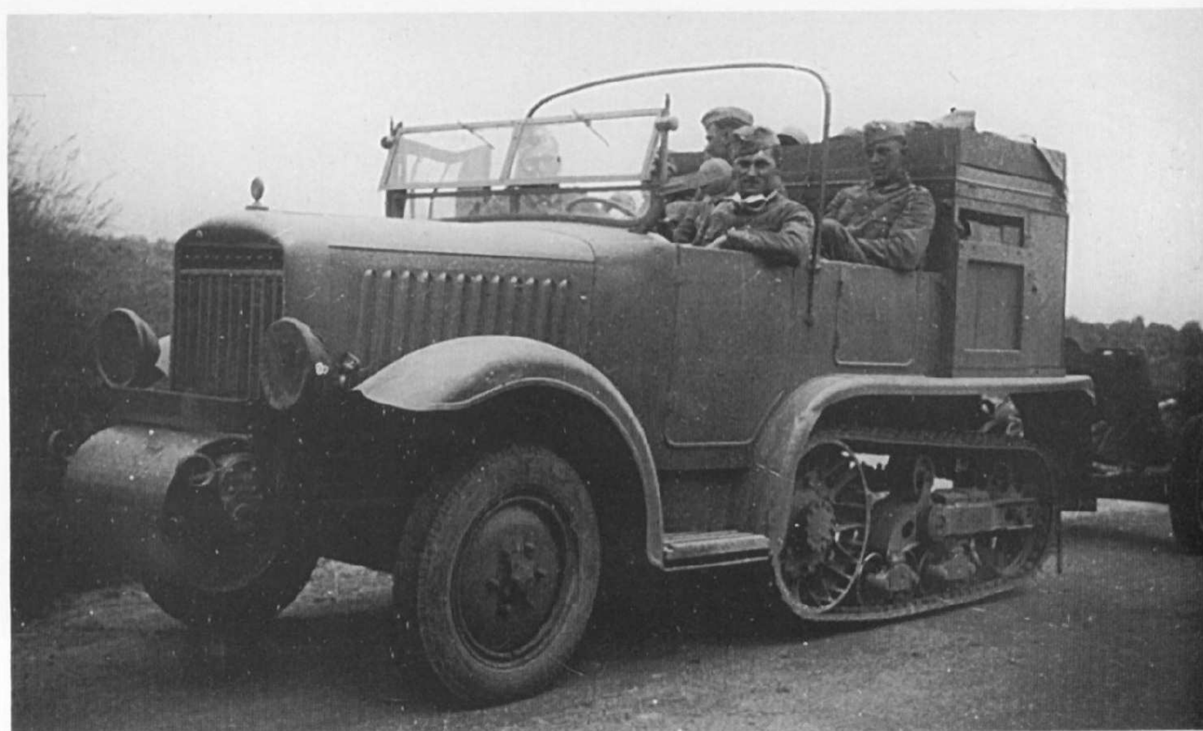
The Unic P 107 304 (f)-frz. towing tractor was used particularly to tow antitank cannons and infantry guns. The picture, taken on the eastern front in July 1941, shows such a towing vehicle towing a 3.7 cm L/45 Panzerjäger cannon.
