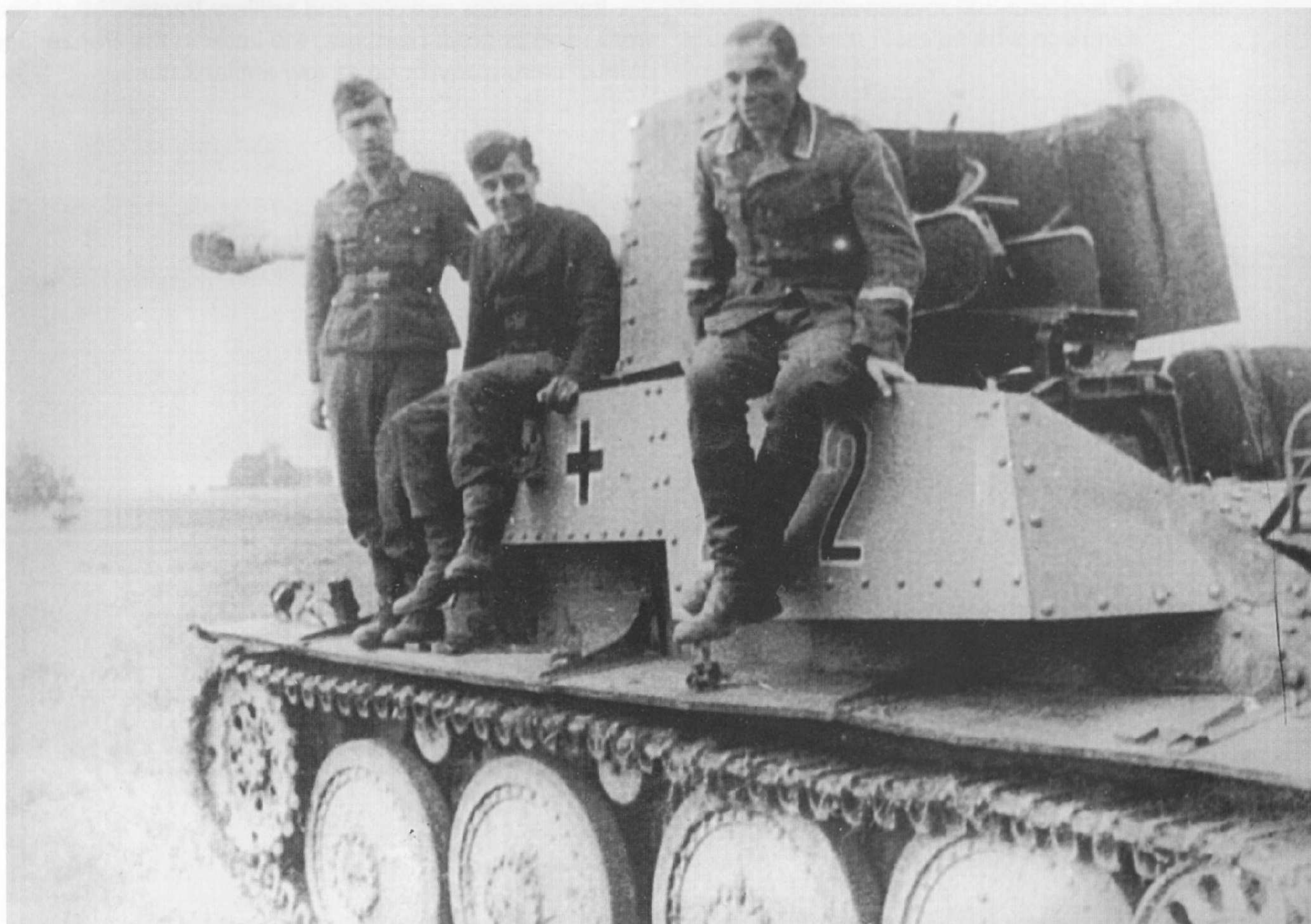
The many captured Russian Field Cannon 36 (designated 7.62 cm Field Cannon 296 (r)-russ. 36-) were reworked to take the ammunition of the German 7.5 cm Panzerjäger Cannon 40 L/46. The new designation was 7.62 cm Panzerjäger Cannon 36. In all, 363 of them were mounted on selected Czech Panzer 38 (t) chassis, beginning in April 1942. The resulting tank destroyer strengthened the antitank forces considerably.
